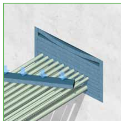
15) Compression of the filling is necessary to obtain stability. For this purpose it is easier to insert a couple of strips instead of sheets. The strips are greased all around with CSD® lubricant.
